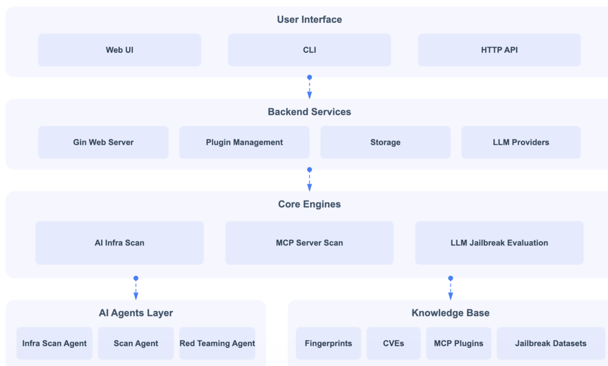
Figure 5 | The distributed server-agent architecture. A user interface (Web UI, CLI, or HTTP API) drives backend services (Gin web server, plugin management, storage, and LLM providers), which in turn invoke the core engines (AI infra scan, MCP server scan, and LLM jailbreak evaluation). The engines draw on an AI-agents layer and a shared knowledge base of fingerprints, CVEs, MCP plugins, and jailbreak datasets.
