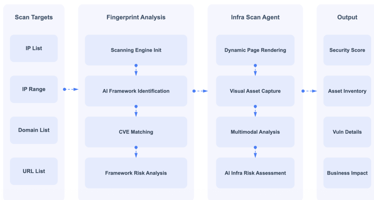
Figure 2 | The infrastructure-scanning pipeline (M1). Targets (IP lists, ranges, domains, or URLs) flow through fingerprint analysis (scanning-engine initialization, AI-framework identification, CVE matching, and framework risk analysis) and an infrastructure-scan agent (dynamic page rendering, visual asset capture, and multimodal risk assessment), producing a security score, an asset inventory, vulnerability details, and a business-impact summary.
